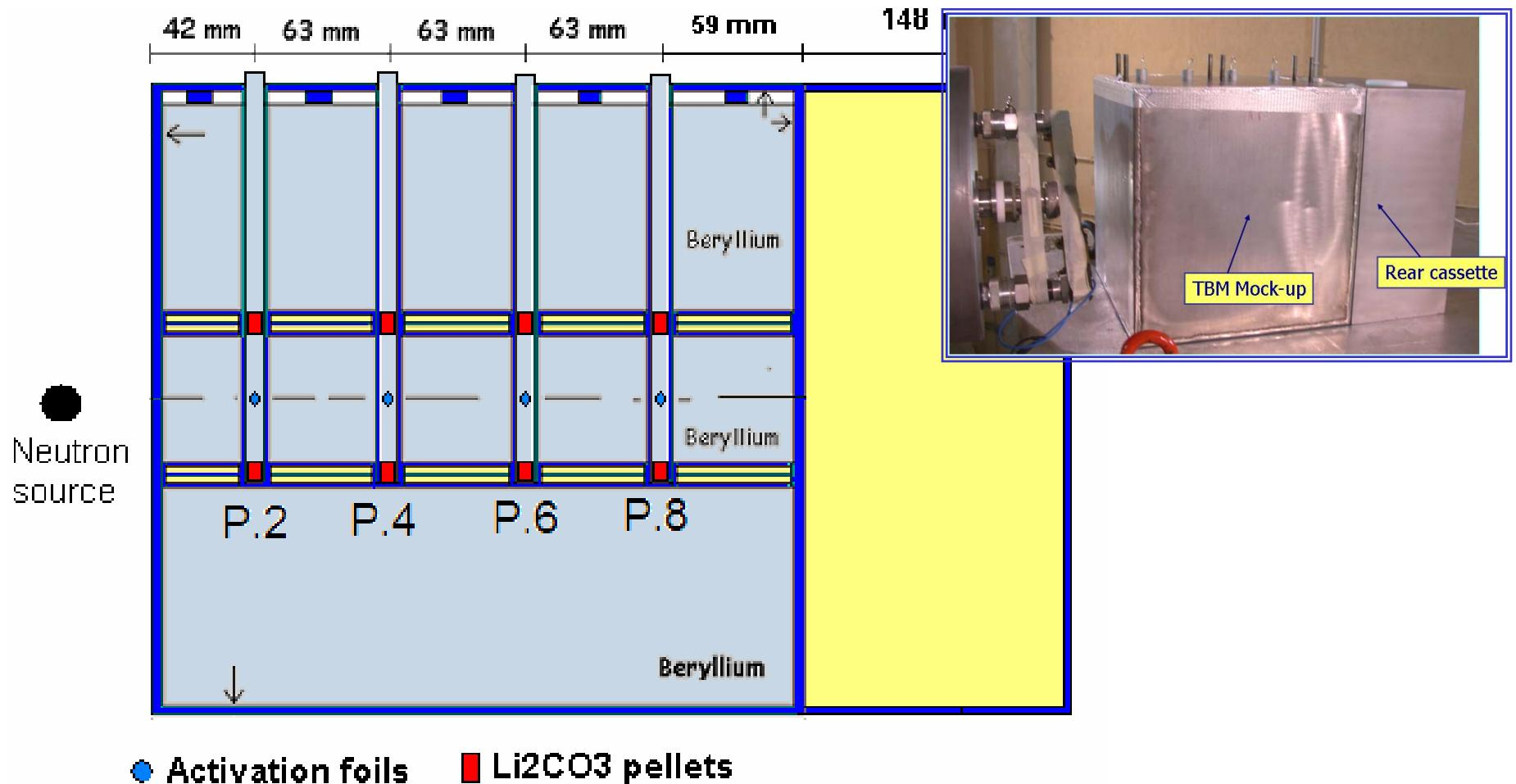
Measurements of tritium production in 4 positions P.2 – P.8 by Li<sub>2</sub>CO<sub>3</sub> pellets (nat. Li)(12 pellet/position) and of the neutron flux in the central Be layer by activation foils
