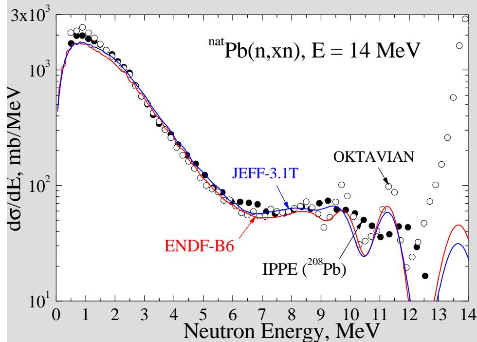
Neutron emission and inelastic for Lead-208
