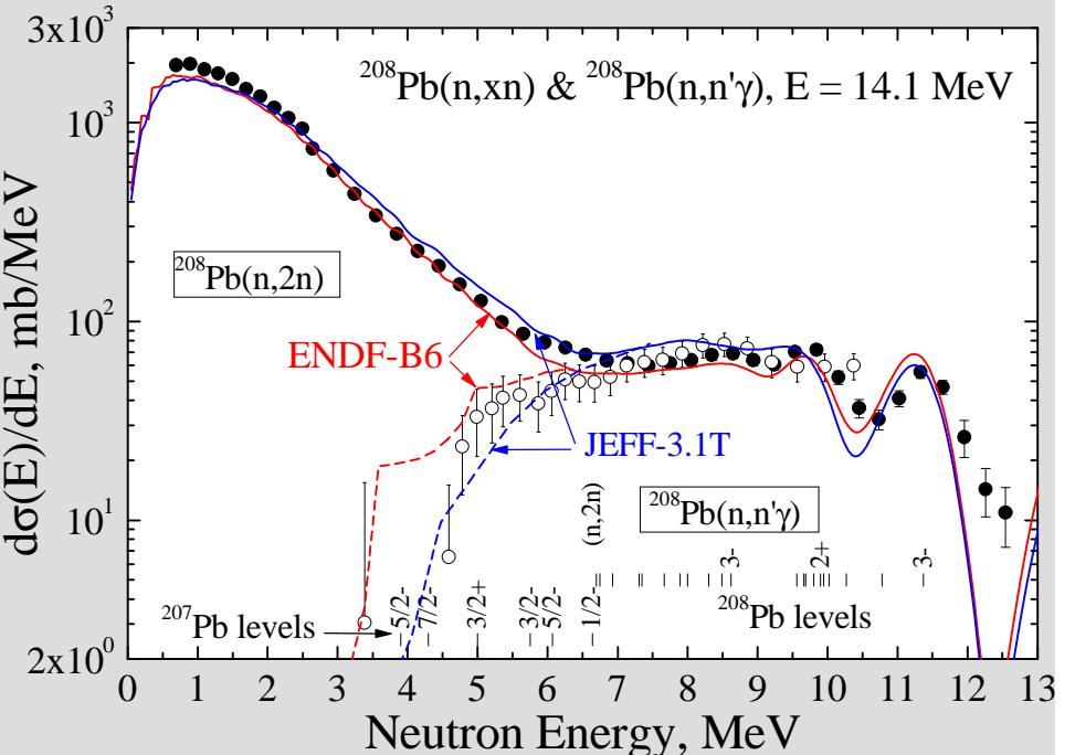
**Findings:** reasonable agreement for energy differential cross section for  ${}^{200}\text{Pb}(n, xn)$  and  ${}^{208}\text{Pb}(n, xn)$  or  ${}^{208}\text{Pb}(n, n'\gamma)$  reactions at 14 MeV
