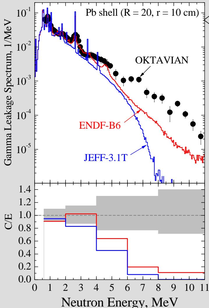
$\gamma$  - Leakage Spectrum from Pb-Shell
