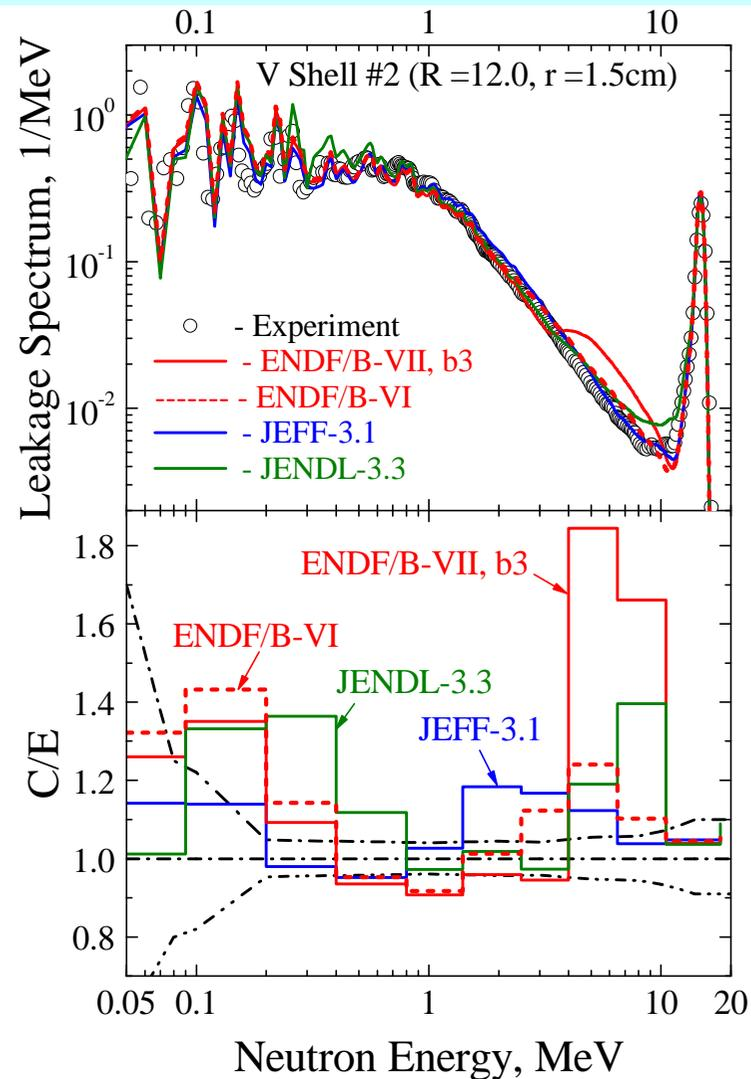
**Findings:** - JEFF-3.1 with higher accuracy (20%) reproduces n-leakage spectra than others
