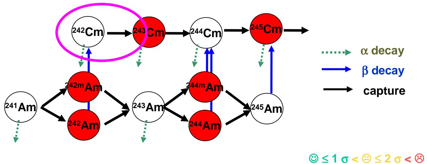
Sample irradiation in T4 {  $^{242}\text{Cm}(\text{n}, \gamma)^{243}\text{Cm} : 22.6 \pm 2 \text{ b}$  }
