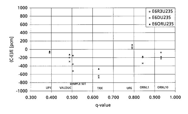
The figure above again excludes the results from the three hard assemblies and is plotted on the same scale as the previous "zoom" figure. Apart from TRX, all results with the new December 1996 ORNL evaluation are within 200 pcm. There is overall improvement over JEF2.2 results even in this range of "q".
