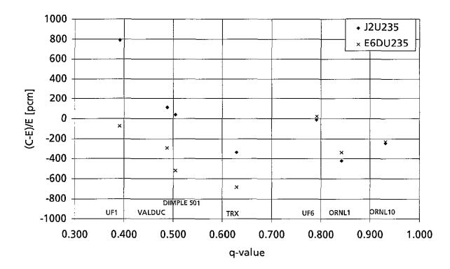
The next figure above "zooms in" on the previous one to show the effect on the softer assemblies. i.e. when the three hard assemblies are removed. All calculations predict  $k_{eff}$  within ~0.5% (500pcm) except with the following experiments:- UF1 and DIMPLES01 with JEF2.2 and TRX with the January 1996 evaluation. There is little difference between evaluations for the soft assemblies (q above 0.8). Unfortunately DIMPLES01 is very important being similar to a PWR in terms of neutron spectrum.
