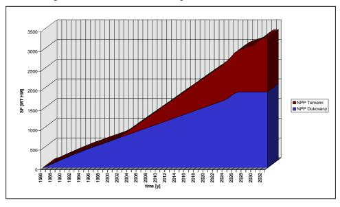
Figure 1. Accumulation of the spent fuel from Czech NPPs
