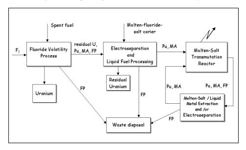
Figure 2. Simplified general scheme of MSTR fuel cycle
