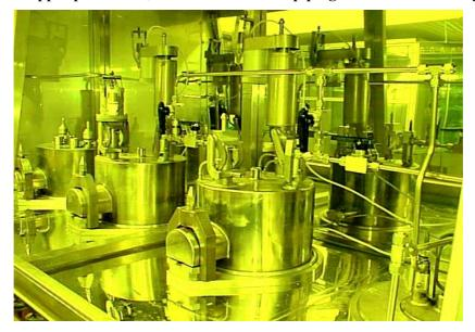
Figure 3. Upper part of UF<sub>6</sub> condensers with the piping and measurement system
