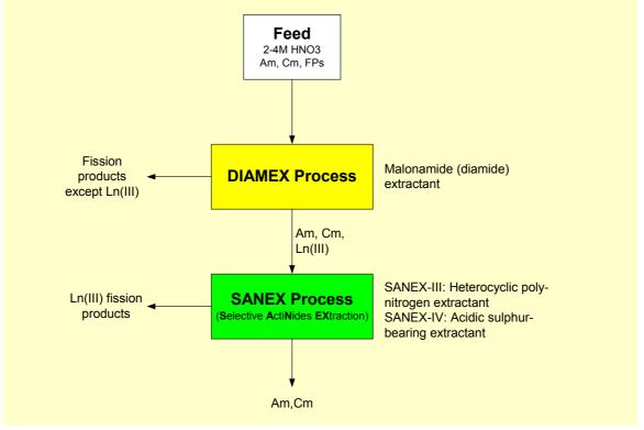
Figure 5. The DIAMEX/SANEX process, among the options being considered in the U.S. programme for the extraction of americium and curium
