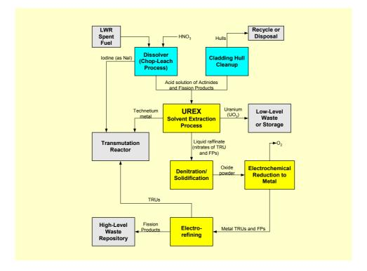
Figure 1. Hybrid aqueous-pyrochemical process (UREX/PYRO-A) for partitioning of spent LWR oxide fuel
