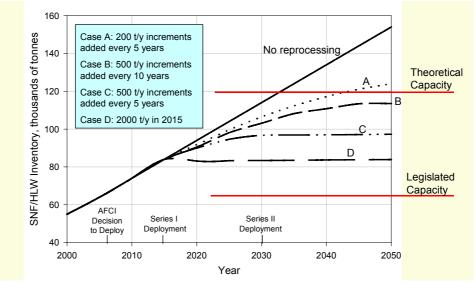
Cases A, B, and C illustrate the serial deployment of smaller-scale plants, while Case D is for a very large plant with 2 000 t per year processing capacity.
