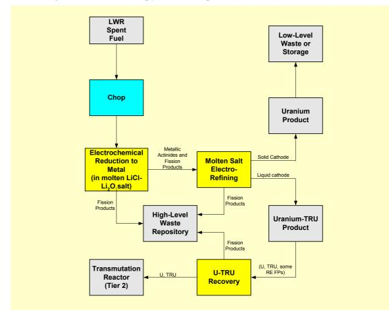
Figure 6. The PYROX pyrochemical process for treatment of LWR oxide fuel
