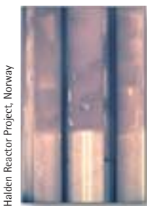
Examples of large (top) and negligible (bottom) crud deposition along a PWR fuel rod after testing in the Halden test reactor.
