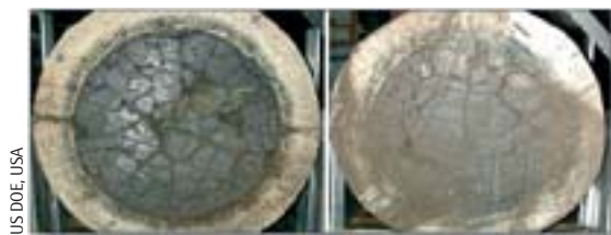
MCCI Project: cross-sections of two water-ingress test sections, obtained after test completion. The tests were run for two compositions containing 8% (left) and 25% (right) concrete respectively in the melt. One can note that the 8% case has more extensive cracking than the 25% case, indicating that the water ingress would be more effective for low concrete content in the melt.
