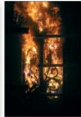
Studying the consequences of an electrical cabinet fire (PICSEL programme, Cadarache, France).
