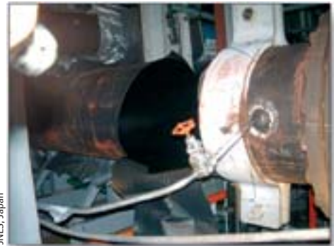
The pipe failure at Mihama Unit 3 in August 2004 led to instructions to review the maintenance records of all of the 22 other PWRs in Japan.
