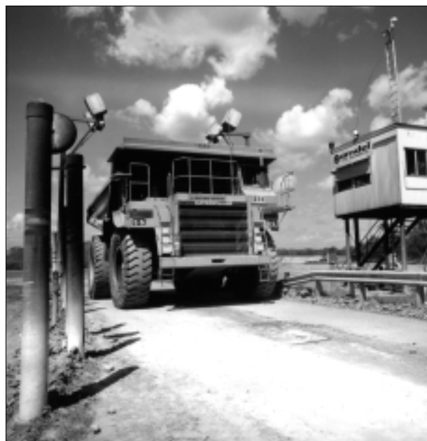
Determining ore grade with a radiometric discriminator at the Ranger Mine in Australia.
