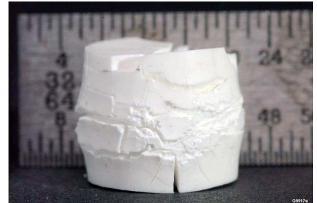
MgO pellet after 3 hr in boiling water
