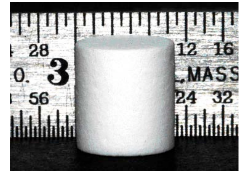
MgO-ZrO 2 pellet after 700 hr in de-ionized water at 300°C
