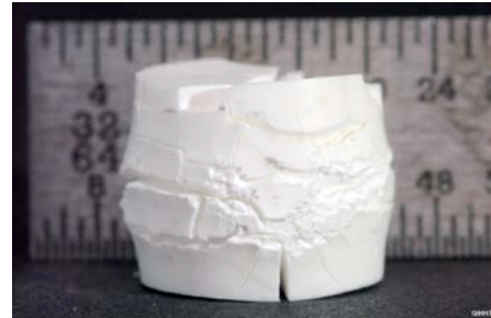
MgO pellet after 3 hr in boiling water
