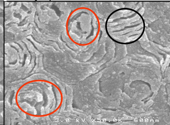
I-PyC polished and etched section
