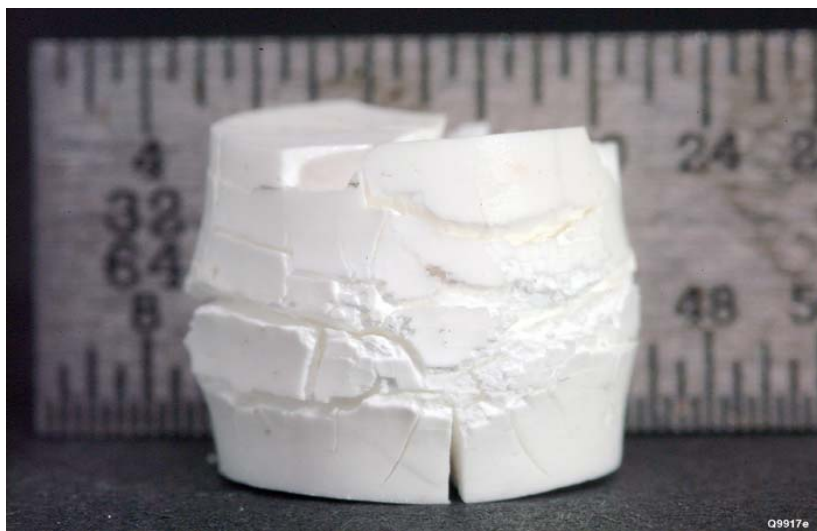
MgO pellet after 3 hr in boiling water
