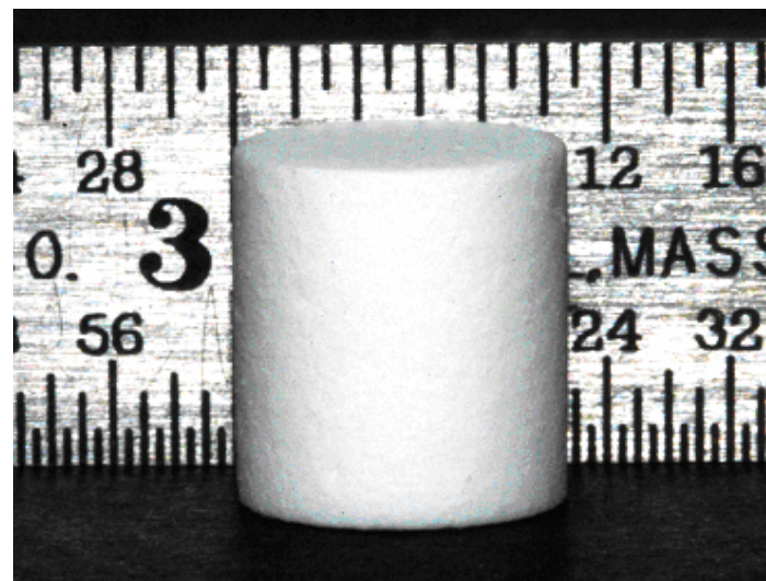
MgO-ZrO 2 pellet after 700 hours in de-ionized water at 300°C
