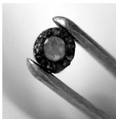
Figure 13. U-Pu-Zr alloy (left) before and (right) after experiment. U-Pu-Zr alloy remaining after experiment was surrounded by dense layer with Zr metal and salt mixture
