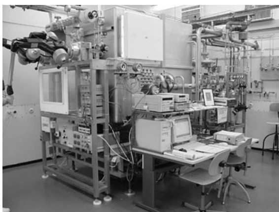
Figure 12. Internal view of the caisson (Electrorefiner operated with manipulator)
