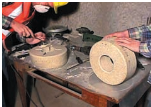
Manufacturing of a bentonite barrier at Mont Terri, Switzerland.
