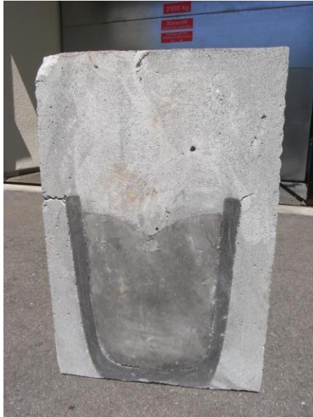
Crucibles filled with Al and placed in a PSI concrete container
