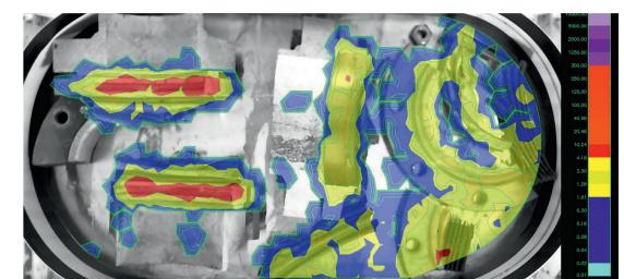
2. Sorting process by γ spectrometry based on Co-60 peak
