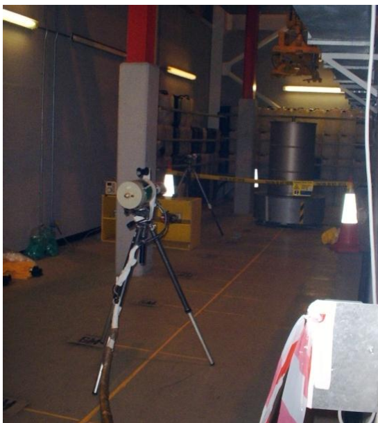
Figure 3: FED Drum Gamma Spectrometry
