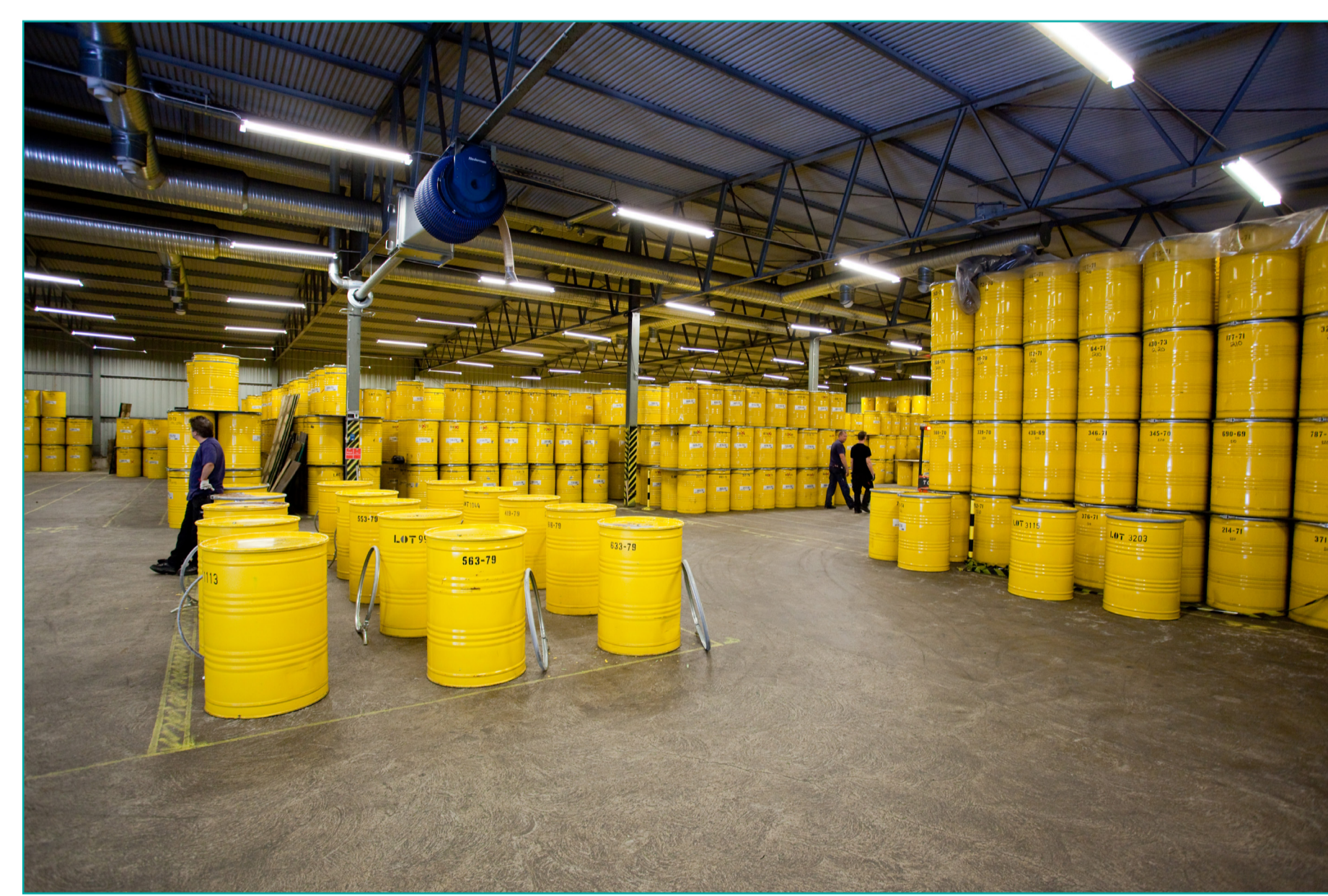
AU facility during the project: Drums were brought forward, id checked, re labeled using age resistant stickers and final contamination check prior to RTR and gamma assay.
