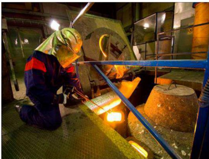
Fig.1. Induction furnace at Studsvik for melting ingots of contaminated metallic low level waste.
