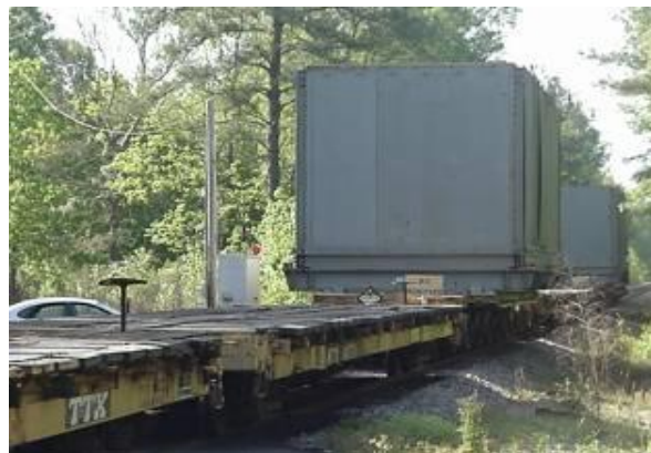
Figure 6 Moving S/G Lower Assembly (with Shielding) to Barge Slip and Via Rail in South Carolina
