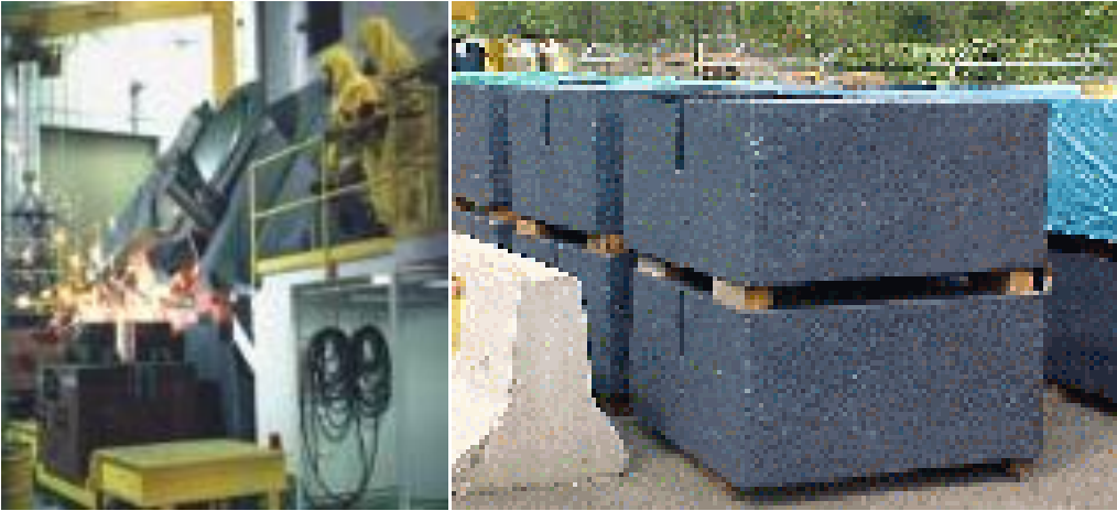
Figure 12 EnergySolutions Metal Melter and Shield Blocks for Recycle
