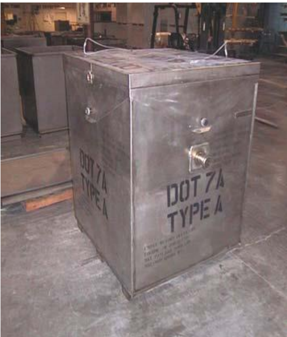
Figure 11 Shielded Shipping Container
