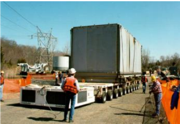
Figure 6 Moving S/G Lower Assembly (with Shielding) to Barge Slip and Via Rail in South Carolina
