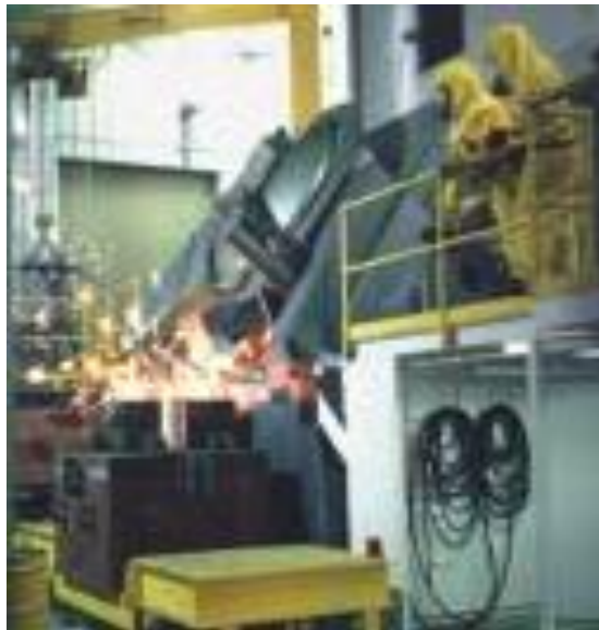
Induction Furnace at EnergySolutions Facility
