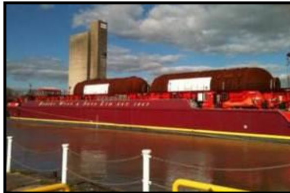
Figure 7 Boilers loaded onto barge at Sharpness
