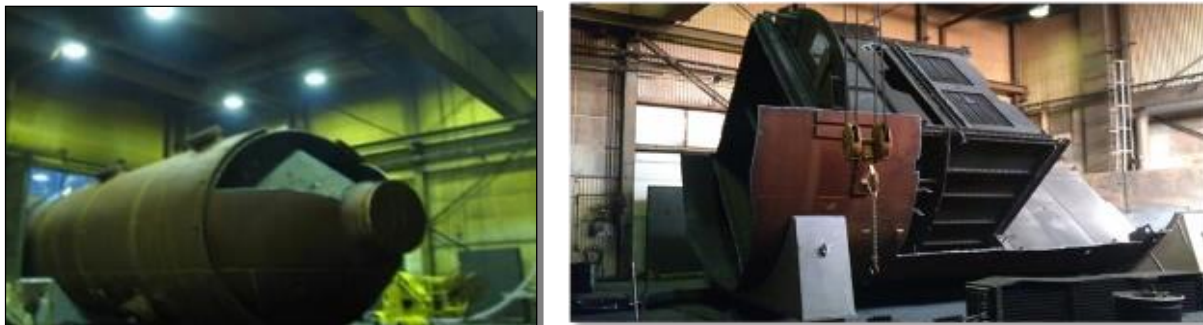
Figure 10 Boiler segmentation in Studsvik treatment facility
