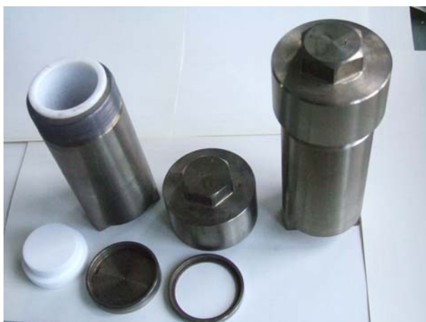
Figure 1: Picture of the equipment used for hydrothermal leaching: Teflon vessels and steel autoclaves
