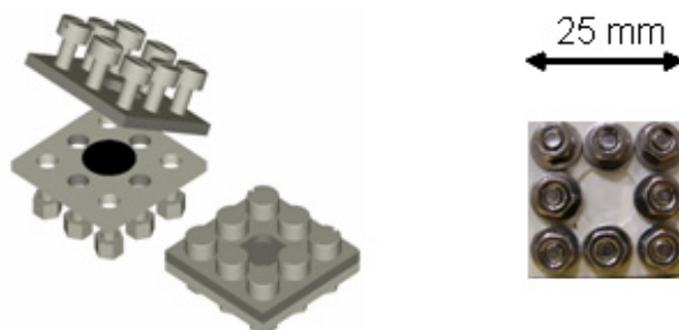
Figure 1: Cell for EXAFS measurements in molten fluorides
