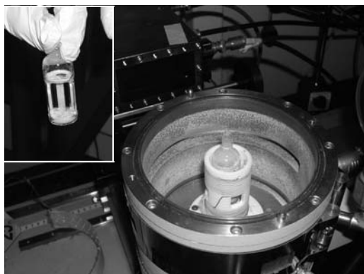
Figure 2: The electric furnace fixed between two ionic chambers at BL27B/PF/KEK. A Ge SSD is located on right-hand side of the furnace.
