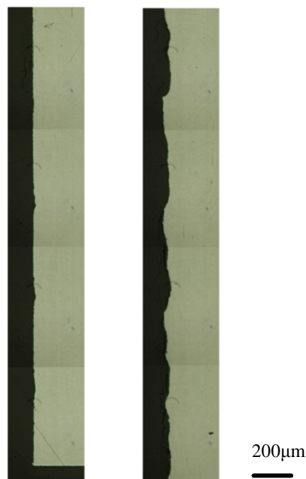
Figure 6: Surfaces of the lower part (left) and the upper part (right) of the test capsules of RbI
