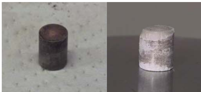
Figure 3: Appearances of CuI (left) and BaI 2 (right) after thermal experiments
