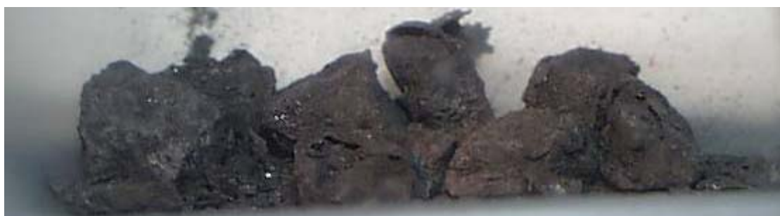
Figure 4: Appearance of U-10Np-29Pu (4.121 g) after the vacuum distillation
