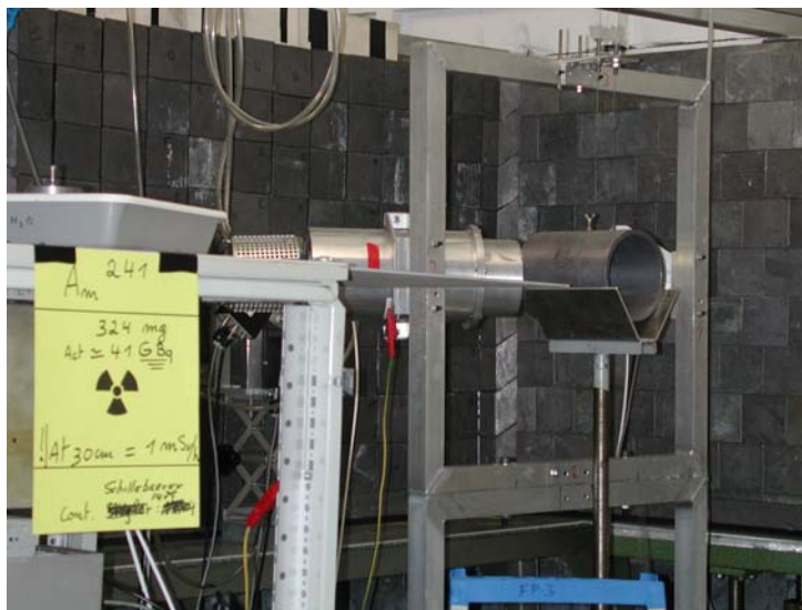
Figure 4: Experimental set-up for the capture measurements
