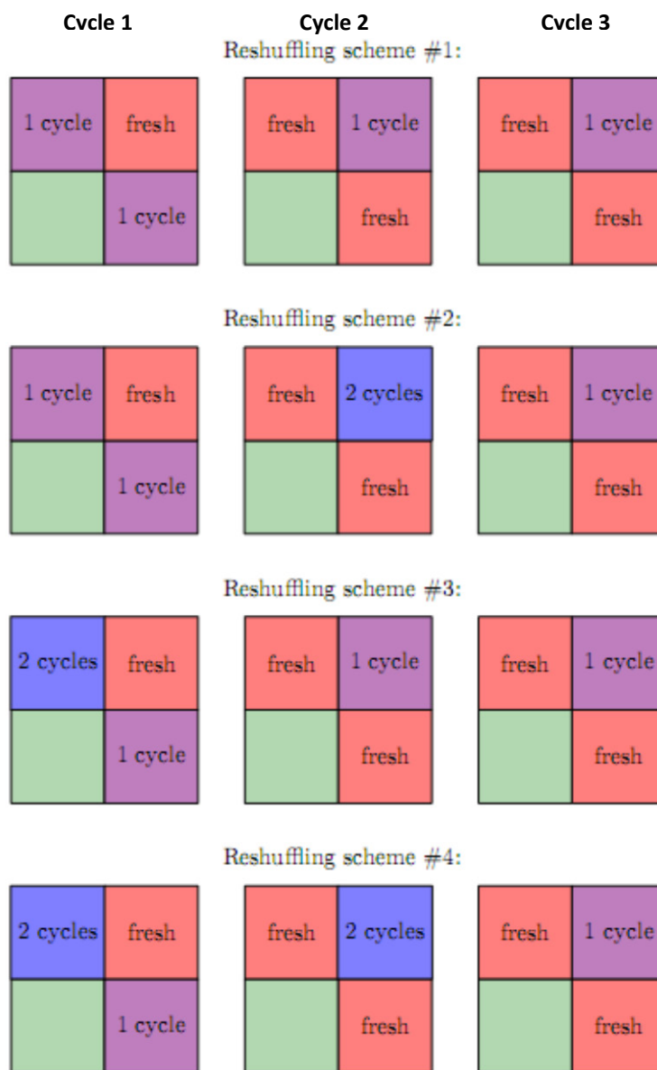
Figure 16: Assembly shuffling schemes showing neighbour assembly initial cycle compositions [124]
